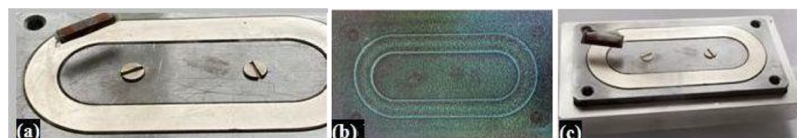
Figure 19. First experiments with an oval-shaped PMG without any gaps ('one-piece' design or non-composite magnet): (a) stable levitation of Sabot #2 ( T \sim 80 K, HTSC-sabot axis along the track); (b) magnetic field mapping by MFV film; (c) stable levitation of Sabot #1 ( T \sim 80 K, HTSC-sabot axis across the track).
