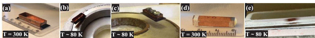
Figure 3. The HTSC-sabots used in the experiments: (a) Sabot #1 (mass is 1.25 g); (b) Sabot #1 with liquid nitrogen inside in the round PMG-1; (c) Sabot #1 levitation with a load capacity of three cylindrical surrogate targets (1.1 g each) in the round PMG-2; (d) Sabot #2 (mass is 1 g) with a polymer foam inside (shown on the right); (e) Sabot #2 acceleration in the inclined linear PMG.
