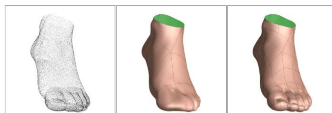
Figure 6. Example of surface reconstruction (Eck et al., 1996). Left: initial point cloud; middle: first NURBS approximation with quadrilateral network with 35 patches and 1.36% maximum error; right: refined network with 285 patches and 0.41% maximum error
