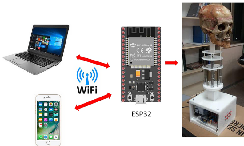
Figure 6. The robot Wi-Fi wireless connection with a smartphone or laptop.
