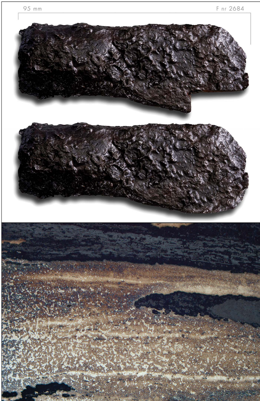
Figure 6. Socketed axe from the Sangis smithing site (Sangis 730) with a multi-layered structure indicating steel. The micrograph cross-section shows light lines indicating welding seams (photograph by S. Nygren © Norrbottens Museum; micrograph by L. Grandin © The Archaeologists, Swedish National Historical Museums).
