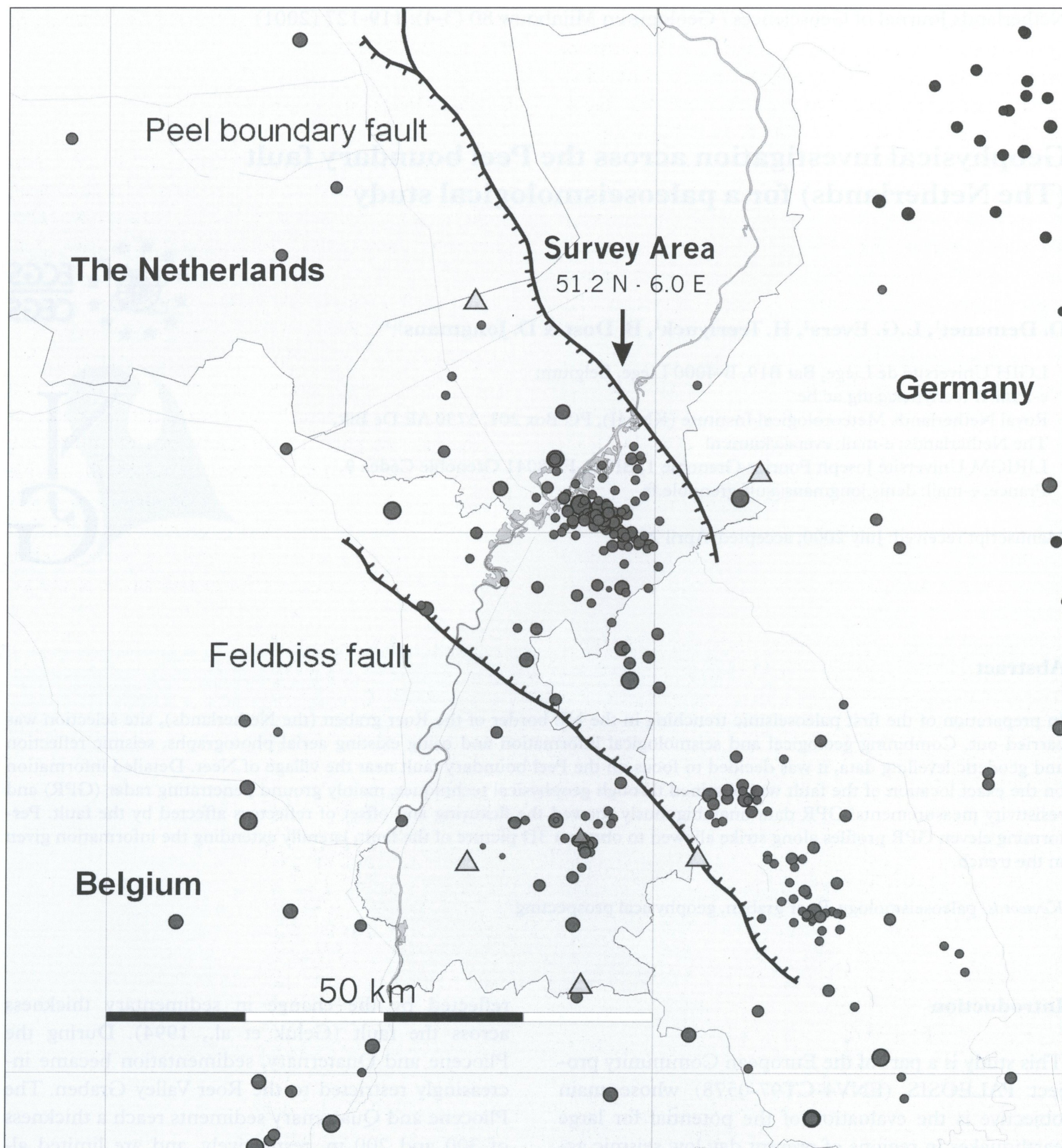
Fig. 1. Overview of seismicity in the Netherlands and surrounding region (1980-2000). The Peel boundary fault is the north-eastern boundary of the Roer Valley Graben while the Feldbiss fault bounds it to the South-west. The dots represent earthquakes and the triangles denote seismological stations.
