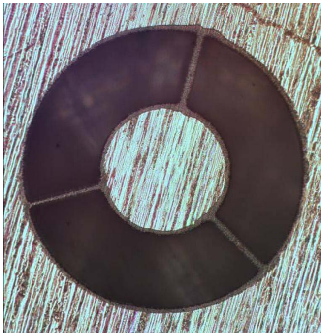
Fig. 1. Optical microscope image of a plasma etched, tantalum annular objective aperture
