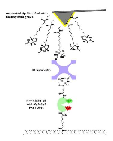
Figure 1. Single-molecule AFM-FRET ultra microscopy, a schematic diagram of one FRET dyes (Donor-Acceptor: Cy3-Cy5) pair labeled HPPK (a kinase) molecule tethered between a glass cover-slip surface and a handle (biotin group plus streptavidin), and a biotin group modified AFM tip. Single-molecule fluorescence photon counting images of the donor (Cy3) and accepter (Cy5) are obtained by donor-acceptor two channel microscopic imaging.
