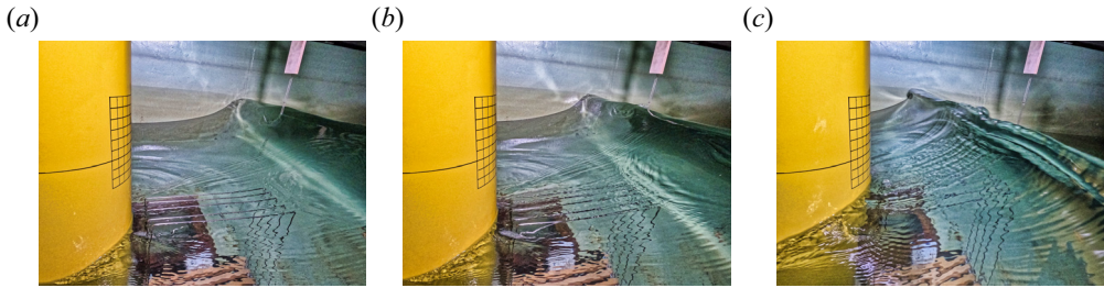
Figure 5. The induction of perturbation by the mechanical perturber and the wave surface: (a) t_0 , (b) t_0 + 3 \Delta t , (c) t_0 + 8 \Delta t .
