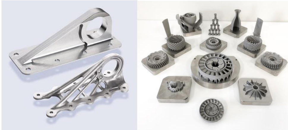
Figure 3a. (left) Two parts with equivalent functionality, which could be used as reference parts to fairly compare impacts of different manufacturing methods ( Airbus Operations GmbH, 2016 ), and Figure 3b. (right) parts with complex interior geometries which are easier to produce by AM ( Aurora Labs Ltd, 2019 ).
