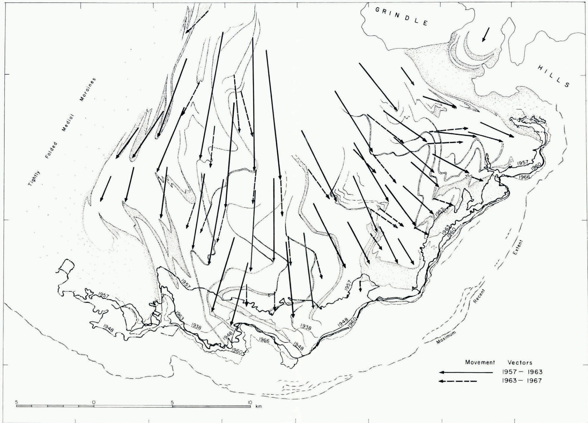
Fig. 4. Map with movement vectors showing the direction and displacement of identifiable debris on Bering Glacier and recent terminal changes. The folded medial moraines are shown in their 1963 positions. Solid arrows denote movement, most of which took place during a surge that ended in 1960; the dashed arrows show the displacements which occurred during the smaller 1965-66 surge. Note the normal radiating patterns of ice flow; there was no evidence of buckling in the piedmont lobe which would lead to the large folded structures present. Changes in the terminal position of the glacier demonstrate alternate advances and retreats that are judged to be due to periodic surging. Fragmentary trim lines and terminal moraines are shown. The maximum recent extent of the glacier in recent centuries is from a map by Miller (1961).
