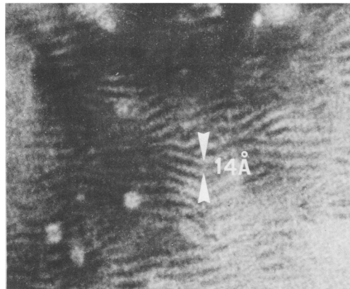
Figure 15. Lattice fringe image of smectite-like zone in a "glauconite" pellet showing many 00 l lattice fringes ( d(001) \sim 14 \text{ \AA} ) altered by numerous edge dislocations. Ion-thinned specimen.
