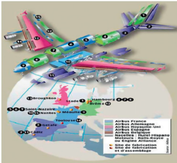
Figure 9 Airbus’s JIT production system.
