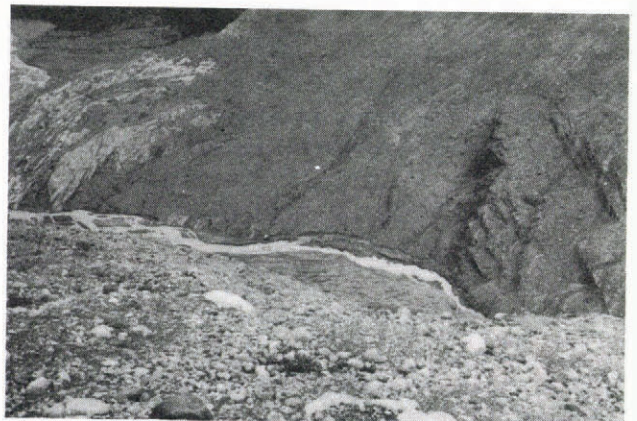
Fig. 9. The gauging site after the landslide and flood event Note the change in position of the survey boulder and the changes in the stream channel.
