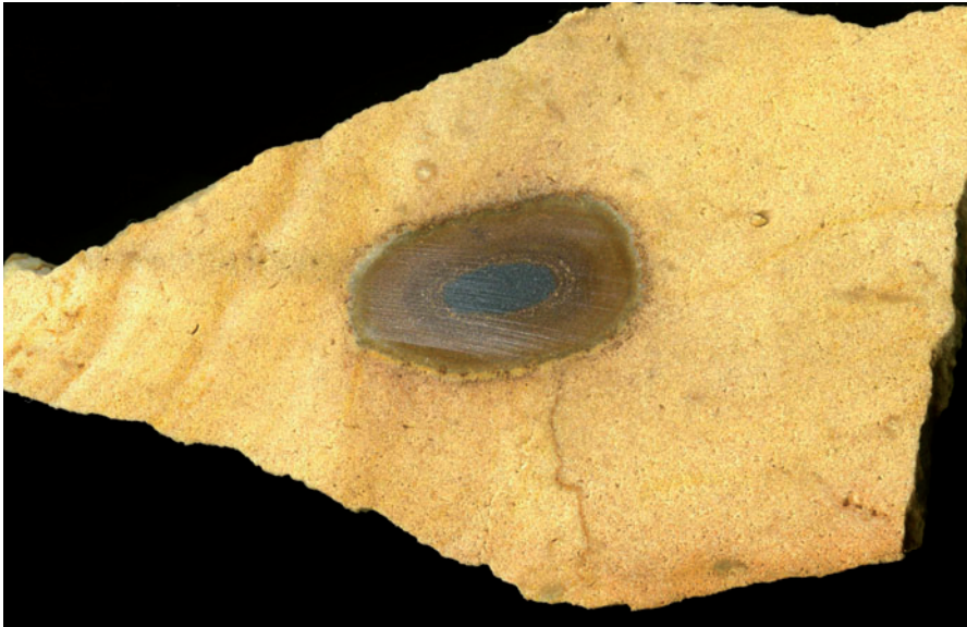
Fig. 5. 'Elst tauw' from the Maurissen sand pit: cut surface in yellowish white (when dry, rather orange yellow when wet) rather dense, medium-grained, silicified calcarenite with large pores, dissolved serpulid with internal fill; vague rusty brown large-scale (almost metric) Liesegang rings; with zoned flint nodule (2 cm diameter) with grey core, dark purplish brown rings with lighter quartz speckles, more homogenous purplish brown mantle with discoloured rim and finally dense caramel brown crust with indentations and patches of rusty brown more porous transition zone to silicified calcarenite. The purplish brown colour is due to disseminated pyrite (R. Meuris Collection).
