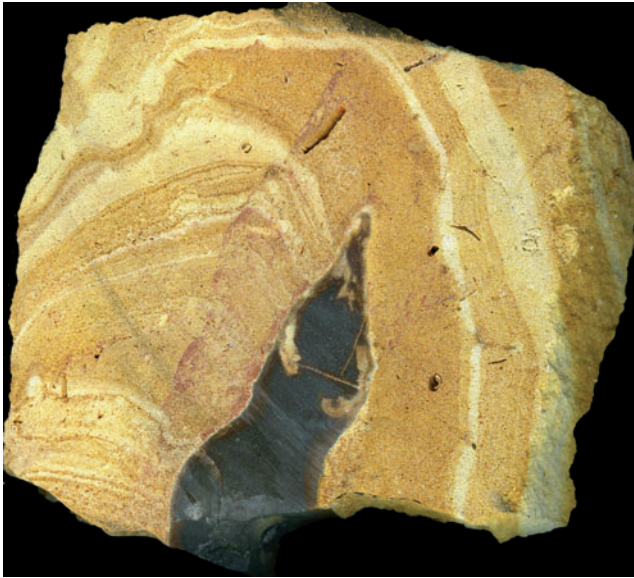
Fig. 7. 'Elst tauw' from the Maurissen sand pit: cut surface (largest diameter 10 cm) in silicified mouldic bioclastic limestone with Liesegang rings crossing flint nodule, brown bands being more porous; flint nodule showing grain texture comparable in size to the surrounding matrix, with outer purplish brown coloured band and whitish front in the silicified calcarenite; reddish oxidation fronts away from the flint (L. Indeherberge Collection).
