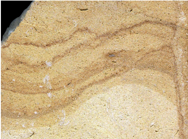
Fig. 9. 'Elst tauw' from St Servatius church at Sluizen: cut surface (width 10 cm) in creamy-white silicified mouldic-bioclasic limestone, still containing calcitic allochems, displaying brown Liesegang rings which concentrate iron and insolubles, possibly developed after extraction (RBINS building stone collection 222).
