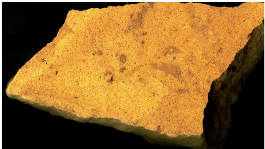
Fig. 6. 'Elst tauw' from the Maurissen sand pit: cut surface (largest diameter 10 cm) in orange brown, strongly porous 'vuggy' silicified calcarenite with frequent moulds of dissolved fossils (thin shells, serpulids, cidarid echinoid), displaying pedogenic weathering (R. Meuris Collection).
