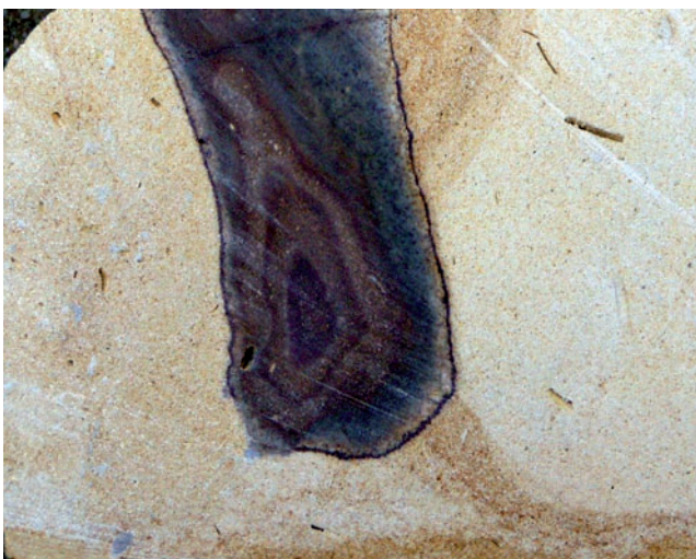
Fig. 10. 'Elst tauw' from St Servatius church at Sluizen: cut surface (width of flint nodule 3 cm) in light yellowish brown silicified mouldic bioclasic limestone containing elongated, purplish zoned flint nodule. Matrix silicification provides strong bond between original flint and surrounding tauw (RBINS building stone collection 222).
