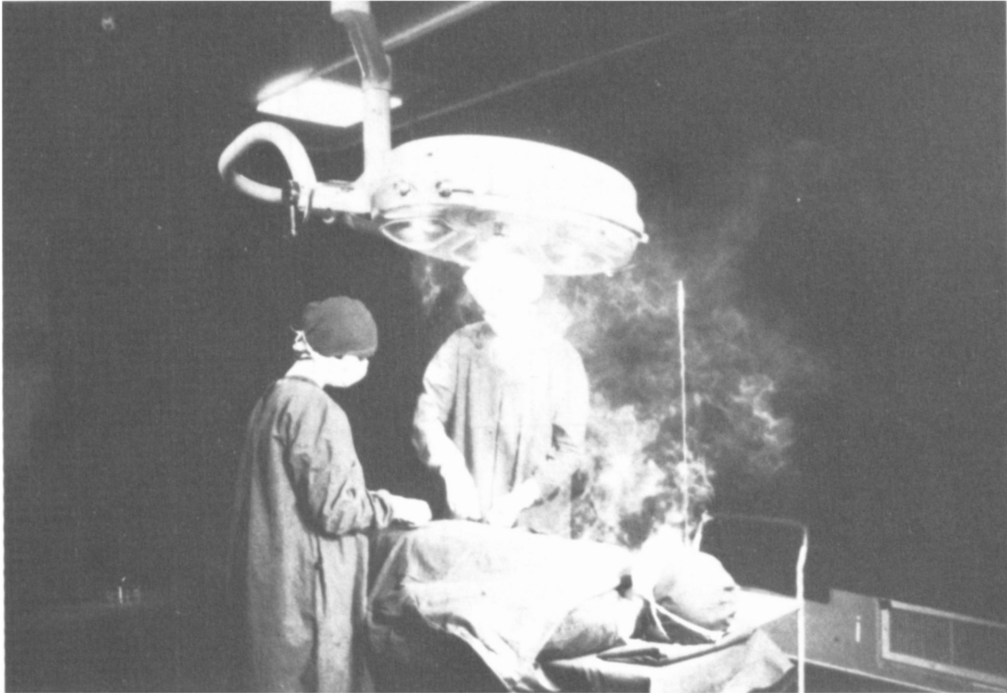
Fig. 2. Dispersion process when smoke was released close to the operating table.
