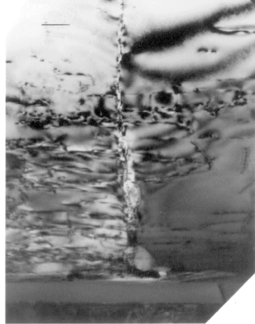
Figure 10. TEM micrograph of a GaN film grown over a silicon nitride mask. The coalescence boundary acted as a nucleation source for horizontally oriented dislocations.
