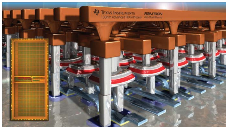
Figure 2. Schematic of the architecture of a 4-Mb ferroelectric random access memory device (from Texas Instruments/Ramtron).
