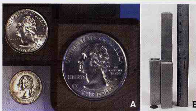
Figure 5. A: Image taken with a 600CL of US quarters on blocks of wood. The image was levels adjusted and sharpened in Adobe Photoshop. The camera was focused on the middle quarter with the Computer iris at f 5.6 and the image taken at an f-stop slightly above "+" (i.e., more than one f-stop above 32, see Fig. 4). Image depth of field/field width is approximately 3.5. B: Side view of the same objects shown in A. Approximately 140 mm (5 1/2 inches) separate each quarter for a total depth of field of more than 280 mm (11 inches).
