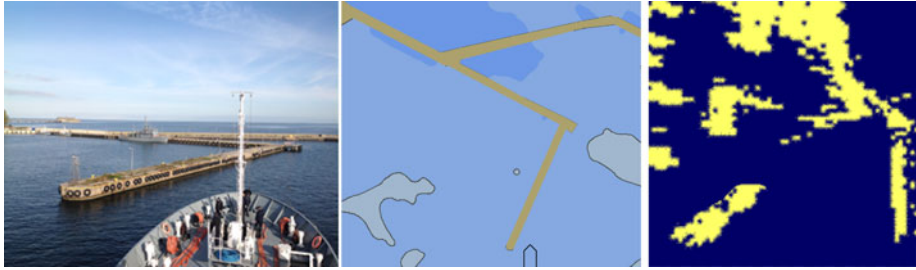
Figure 1. Left to right, images of coastline as seen from a ship with a perspective camera, the same coastline as seen on a navigational chart, and as seen by radar.
