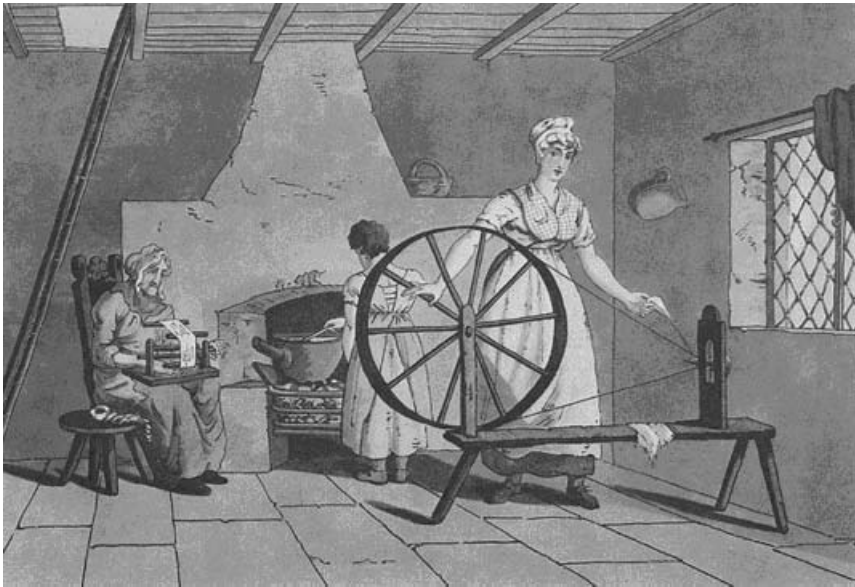
Figure 2. This watercolor shows a Yorkshire spinner at her great wheel. The seated woman on the left is reeling the yarn into hanks.
