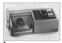
Automatic Sample Notcher: Atlas Polymer Evaluation Products' automatic sample notcher enables users to simultaneously notch as many as 12 0.32-cm-thick specimens. Features include automatic feed rate and cutter speed control. Cutter speed is variable in the range of 0–137 m/min and feed rate is variable within 0–16 cm/min. An air jet applied to the single-tooth rotary cutter removes chips and cools the cutting blade, preventing notch melt-back. A notch verification tester is included.
