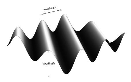
A typical wave, with the definition of two terms for describing the wave.
