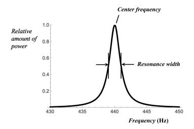
A typical resonance curve. The ratio of the center frequency to the width of the resonance is called its Q-factor.
