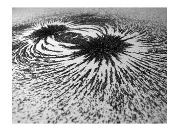
Magnetic field lines from a bar magnet (placed under the board) seen in the alignment of small iron filings. (Windell H. Oskay (www.evilmadscientist.com).)
