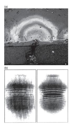
Pictures of interference in the real world. (a) Fringes of light reflected from oil, caused by the interference of light from the top surface and the bottom surface of the oil, with slight thickness variations of the oil (Creative Commons Attribution – Share Alike 2.5 Generic). (b) Interference patterns of matter waves composed of whole atoms, measured at very low temperature. From Andrews 1997.
