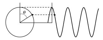
The phase of a wave equated to the position of a clock hand. The angle  $\theta$  is the *phase angle* corresponding to a point in the cycle.
