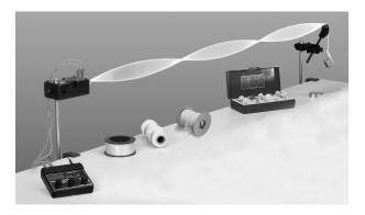
A vibrational resonance of a string produced by an oscillator at one end. The frequency is such that three half-wavelengths fit exactly into the available space. (Greg Severn, University of San Diego.)
