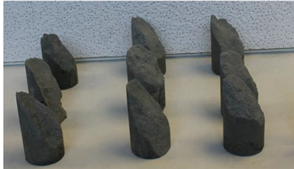
Figure 2. Broken backfill samples after performing uniaxial compressive strength test
