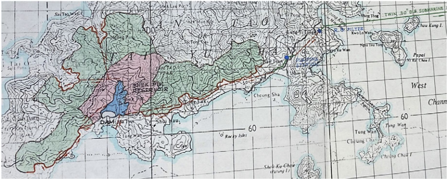
Figure 3. Map (1967) showing the direct (pink) and indirect (green) catchwater-and-tunnel system spanning out from the Shek Pik Reservoir.
