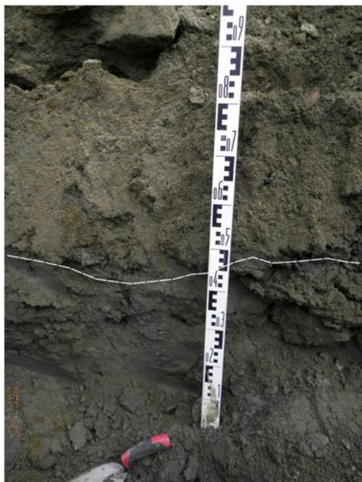
**Figure 10.** Dingle Sand overlying Vestfold Beds in excavator pit CDPEP03 (pit location in Fig. 2). White line follows the contact between units.
