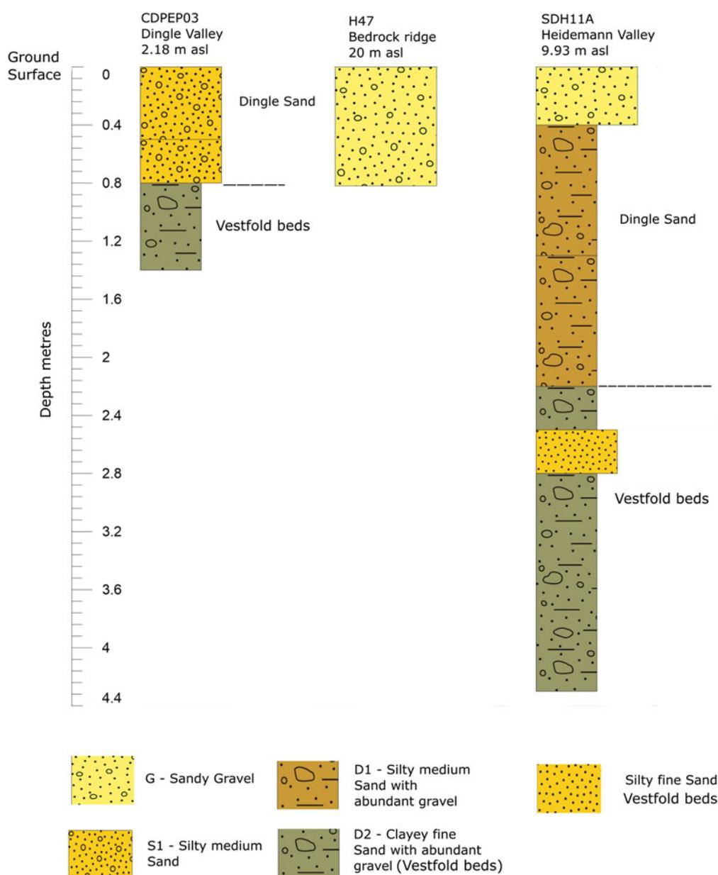
**Figure 4.** Examples of Dingle Sand overlying Vestfold Beds in an excavator pit (CDPEP03), hand pit (H47) and sonic drill core (SDH11A). Sample locations are in Fig. 2. asl = above sea level.
